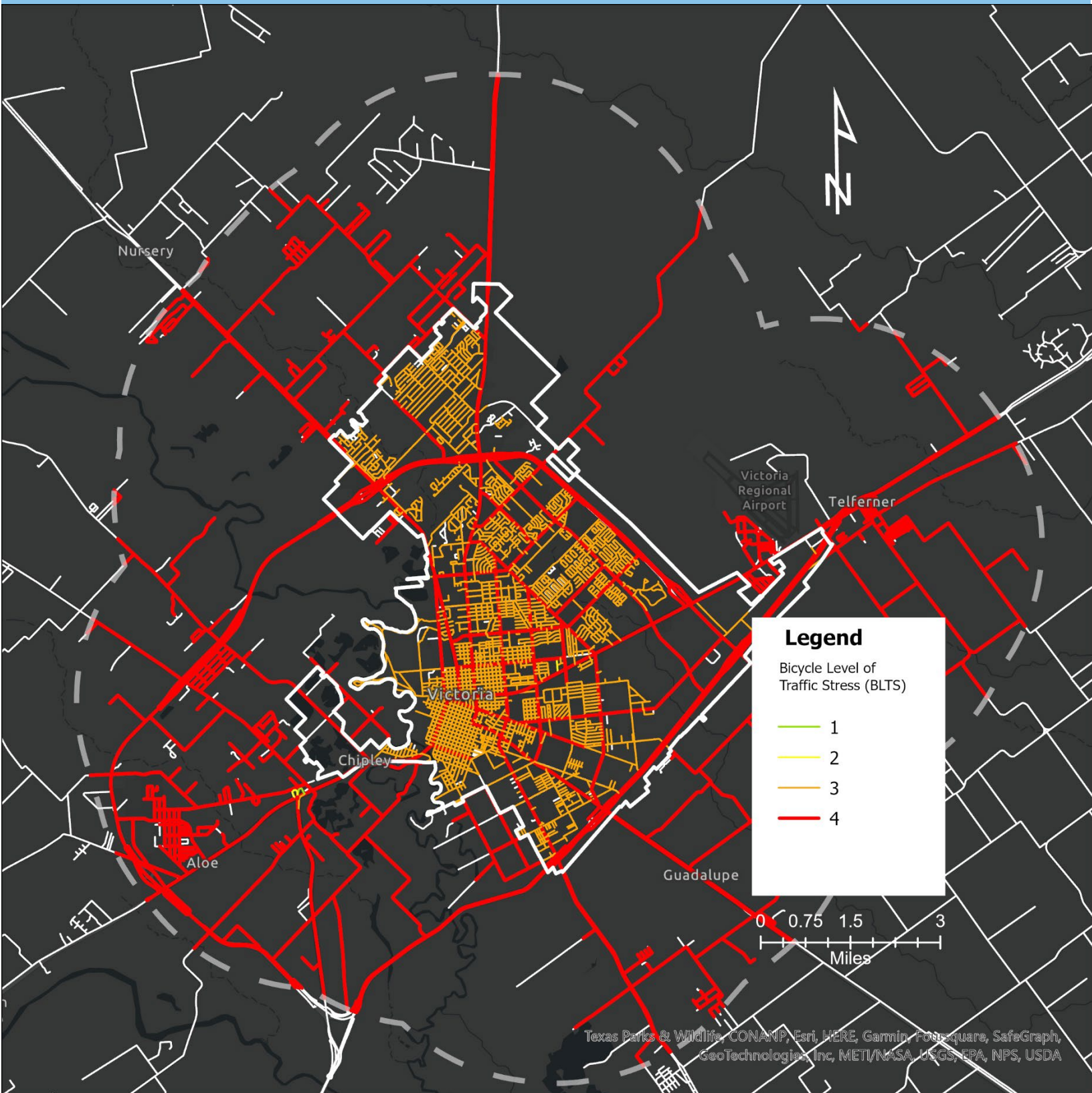
FIGURE 3. BICYCLE LEVEL OF TRAFFIC STRESS (BLTS) ANALYSIS RESULTS
